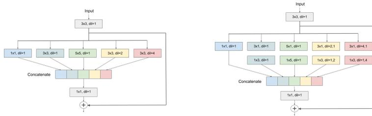
**Fig. 1.** Proposed module which extends inception modules. The module on the left employs standard convolutions while the module on the right adopts the idea of asymmetric convolutions [4].
